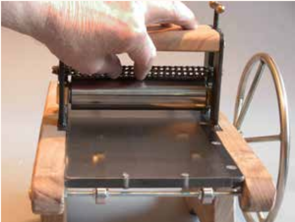
The chain should not be taught, but slightly loose or else the pressure screws will be hard to turn or jerky feeling. The adjustment was made correctly at the factory.
