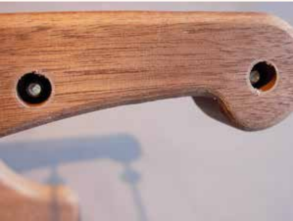
Turn the threaded cross tie rod until about 1/8" can be seen coming through the recessed holes. Start a brass barrel cap nut on this end, holding the threaded rod with the vinyl finger gripper so it doesn't turn with the brass barrel nut.
