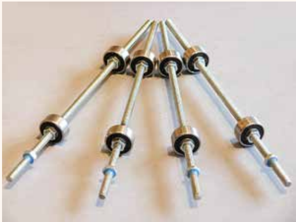
Four threaded steel cross-tie rods have “passive” ends with jam nuts (and an active end without jam nuts). These fit in the holes in both the wood side pieces.
