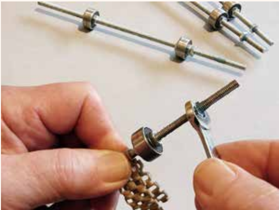
Run the jam nuts all the way to the bearings. When assembling the two sides space is needed for the next step. When the other wood side is fitted, then this jam nut returns to within about 7/8” from the end of the rod.
