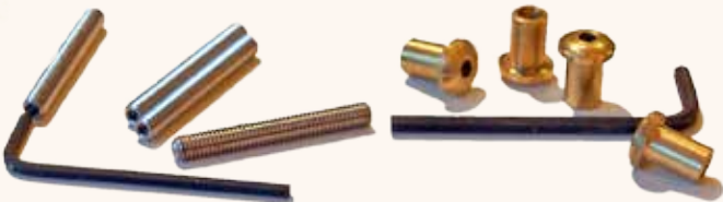
Threaded 1 1/2" long set screws go into the threaded holes of the hood to be screwed in with the 3/32" hex key until about 1/8" extends out for the brass barrel cap nuts.
