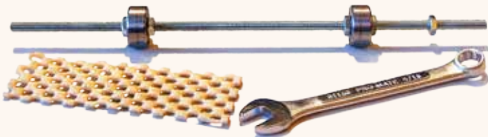
On the passive wood side, which is marked with a P, insert the end of the threaded cross tie rods through the holes. The threaded rod slips in these holes freely because these are not threaded. Be sure it is the end with the jam nut (which had been run up next to the bearing, providing space).
