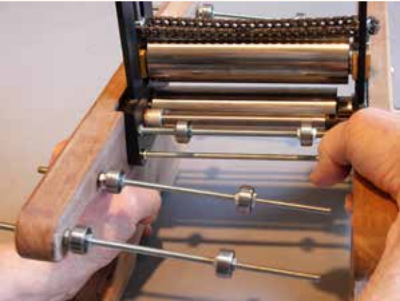
With the jam nuts moved to the bearings, fit the passive side piece on the four threaded cross tie rods of the core. Start the passive side's brass barrel cap nuts.
