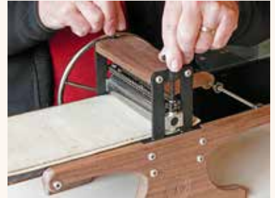
Turn the pressure screws clock-wise to tighten. The illustration shows the felt blankets are under the roller while setting the pressure, using two hands so the chain is not stressed. It is best to load the press with the bed out to the left (facing the wheel, active side of the press) unlike the photo above where the bed is extended to the user's right, the wrong way.
