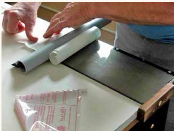
With one end against a stop, tape the covering on the other end to the tabletop with the contact paper reading-side down. Turn back the vinyl, and start to peel the backing away about two inches. With two hands, press and drag the squeegee and peel at the same time all the way to the end of the bed.
