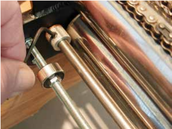
The retaining collar has the simple purpose of keeping the driving shaft in the exact position it was when the core was assembled, and should never need attention. It's shown here only for the user's edification.
