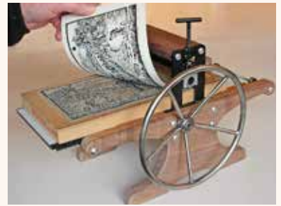
Type-high means that the printing block is the same as moveable type from traditional letterpress printing. Mounted linoleum is sold by companies such as Speedball. The illustration shows a full-size, 6" X 12" block almost the same size as the press bed.
