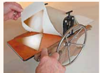
Pochoir printing uses a stencil, shown here as a triangle-shaped window cut in copper, and placed over a rolled ink gradation on a plate done with a brayer. The color only prints through the window.
