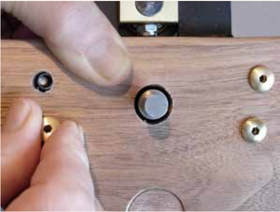
Start the brass barrel cap nuts being sure they are started straight to avoid stripping the threads. Make them finger tight.
