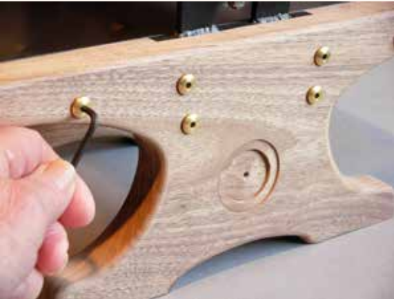
Brass barrel cap nuts fit the threaded screws and are tightened with the 1/8" hex key included with the press. Do not use great force on cap nuts - merely make them snug against the wood.
