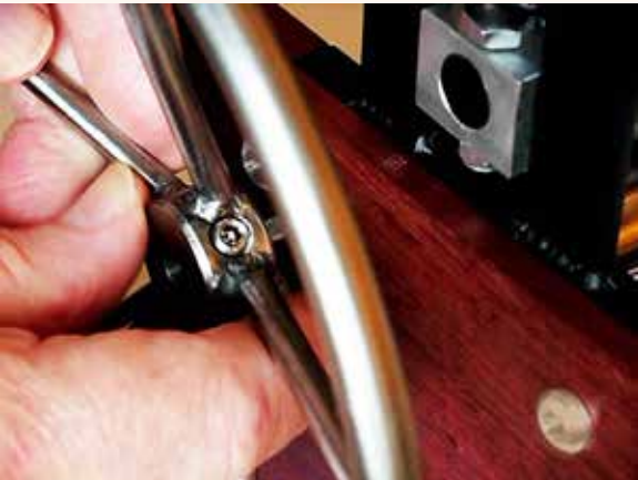
With the set screw loose so it won't catch on the shaft end, align it with the shaft's flat spot and press it on far enough that the set screw will settle on that spot.
