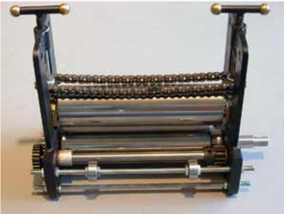
The core of the press has a hood, and it was custom fitted to the core. The length of the core is precisely correct for proper tension of the chain.
