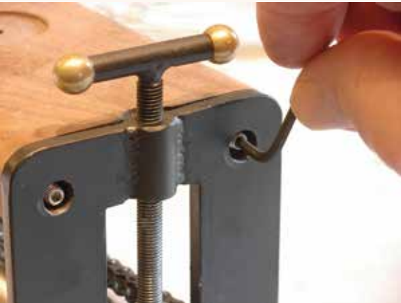
Threaded 1 1/2" long set screws go into the threaded holes of the hood to be screwed in with the 3/32" hex key until about 1/8" extends out for the brass barrel cap nuts.
