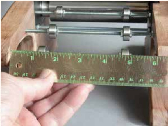
Jam nuts inside the steel core and on the passive side piece determine the slightly wider than 6" space for the bed. Jam nuts in the core should not need to be changed as they were set at the factory.
