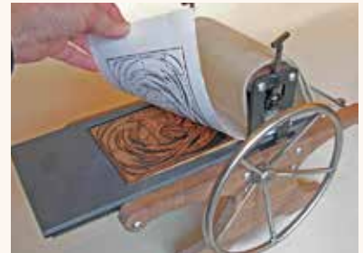
Quarter-inch plywood, or laminated wood, fits in the chase. SafeTKut and acrylic plates plus numerous other block making materials exist, including collagraphs, can be used in the chase if they are 1/4" thick.
