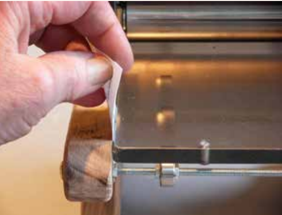
The space between the bed and the side piece needs to be only enough to allow free movement. In the photo, a business card fits in the space between side piece and bed.
