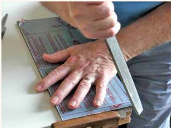
Filing corners and edges of a new bed, as its done at the factory, because they were sharp when newly cut from sheets.
