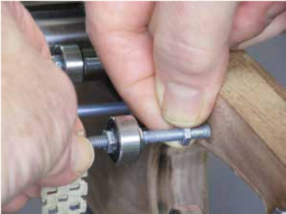
Turn the jam nuts in the passive side to snug against the wood. Use the vinyl finger gripper pad to help hold the threaded rod and prevent its turning.
