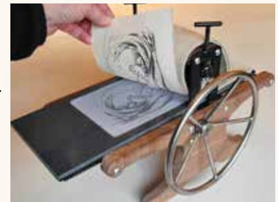
Planographic printing uses polyester plates and vitreography (waterless lithography) uses either quarter-inch ground plate glass or frosted Mylar prepared so that a silicon mask keeps non-printing areas free of ink.
