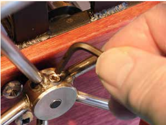
The illustration shows the larger, 1/8" hex key in the set screw on the driving wheel. The set screw was aligned with a flat place on the shaft.
