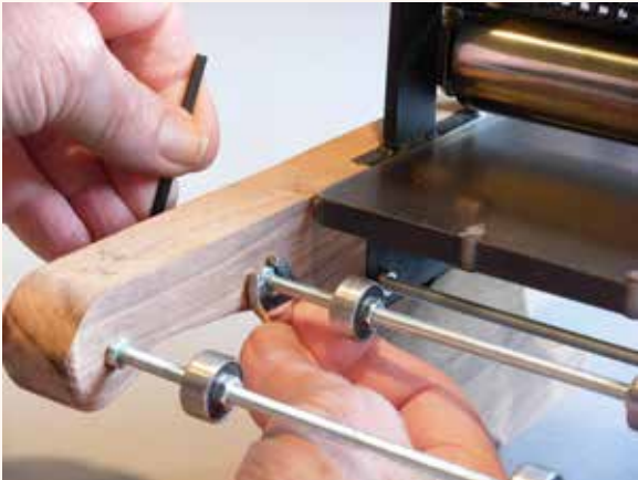
The open end of the 5/16" combination wrench fits the jam nuts on the threaded rod cross-ties on the passive side of the press. The jam nut allows fine adjustment of the space between the bed and the wood side piece - working in union with the brass barrel cap nut on the outside of the wood..
