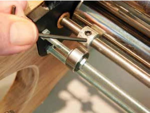
The aluminum retaining collar, located on the passive end of the driving shaft, is shown with the set screw loosened to point out it has only one set screw and no dimple on the shaft like those for the spur gear.
