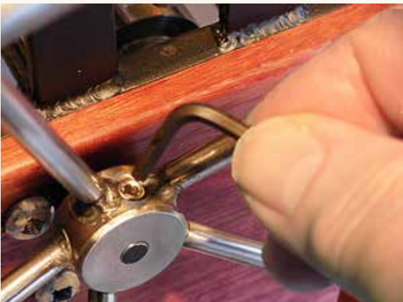
The 1/8" hex key is for tightening the set screw, setting it well into the flat spot so it "bites" into the steel and won't loosen. Check it occasionally to be sure it stays tight.
