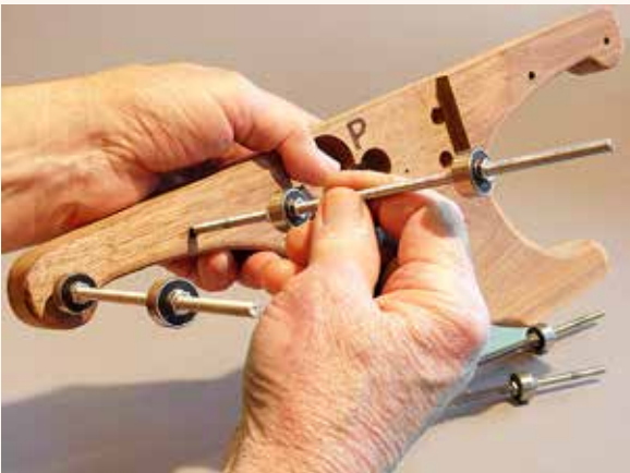
On the passive wood side, which is marked with a P, insert the end of the threaded cross tie rods through the holes. The threaded rod slips in these holes freely because these are not threaded. Be sure it is the end with the jam nut (which had been run up next to the bearing, providing space).
