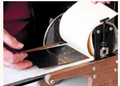
Put a piece of damp newsprint under the plate first, then put the plate on this damp paper so it is less likely to slide or be "bull-dozed" ahead of the roller.
