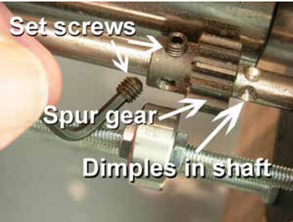
The spur gear has two set screws which are made of hardened steel, and the shaft has two “dimples” drilled in it where the set screws are seated.
