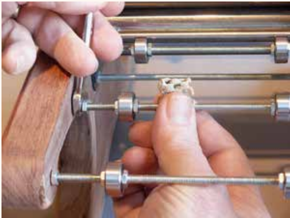
Turn the jam nuts back out to the wood and secure the cap nut and jam nut together. The space between the two wood side pieces should measure a little over 6" - where the press bed will fit. There will be steps for final adjustment of this space in the finished press.
