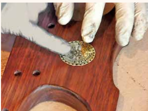
Inset spaces have been cut in for the three round badges. See a later page to see how the badges were made with the laser transfer method - a method that is good for making copper and brass etched printing plates, too. Two-part epoxy glue is best for keeping the badge in place. Clean the metal back with alcohol for best results.
