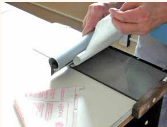
A window-washer-style squeegee is ideal to help avoid bubbles. If bubbles are trapped, make a tiny hole in the bubble and press out the trapped air. Trim the excess all around the bed.
