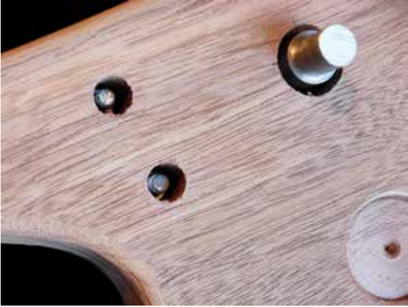
When the active side piece is on, about 1/8" can be seen which has passed into the recessed holes.
