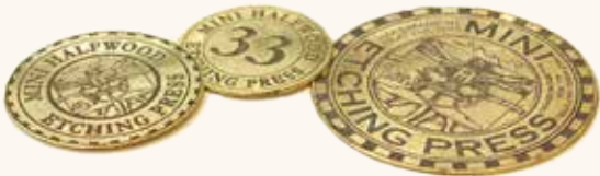
Inset spaces have been cut in for the three round badges. See a later page to see how the badges were made with the laser transfer method - a method that is good for making copper and brass etched printing plates, too. Two-part epoxy glue is best for keeping the badge in place. Clean the metal back with alcohol for best results.
