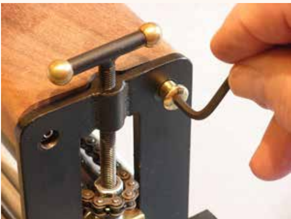
Brass barrel cap nuts fit the long threaded set screws ready to be tightened with the 1/8" hex key.
