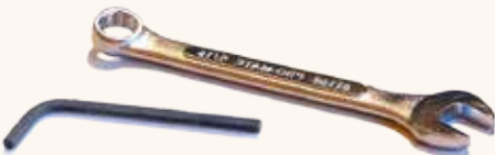
The open end of the 5/16" combination wrench fits the jam nuts on the threaded rod cross-ties on the passive side of the press. The jam nut allows fine adjustment of the space between the bed and the wood side piece - working in union with the brass barrel cap nut on the outside of the wood..
