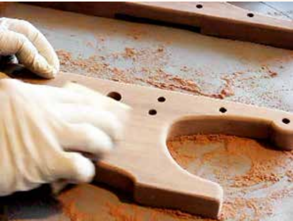
Rasp away rough edges and sand before staining or oiling, starting with coarse sandpaper, graduating to 220 or finer, and then use 000 steel wool to polish.
