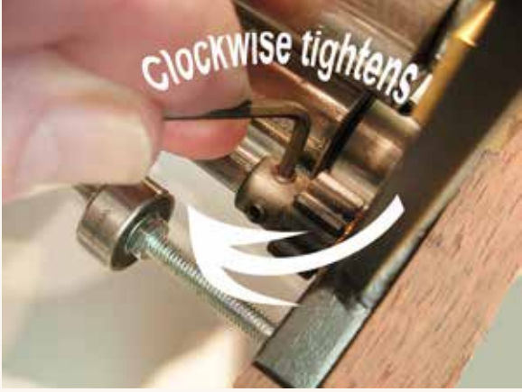
The set screws on the spur gear were tightend at the factory and do not require the user to do this, but checking tightness with the 3/32 hex key is a good idea.
