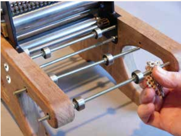
Turn the threaded cross tie rods into the active side piece holes, which are threaded (unlike those in the passive side piece).
