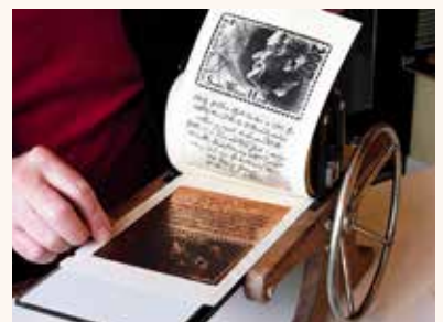
A damp piece of newsprint under the plate, the same size as the printing paper, also helps to align the margins and keeps the margins of the printing paper clean.
